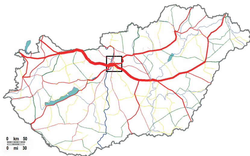
Figure 9: The maximal possible traffic on paths with minimal travel time between the border crossings Note: The thickness of the lines is proportional to the traffic on them. Red: electrified lines with traffic; pink: electrified lines with no traffic; green: unelectrified lines with traffic; yellow: unelectrified lines with no traffic. Source: TÓTH 2019
