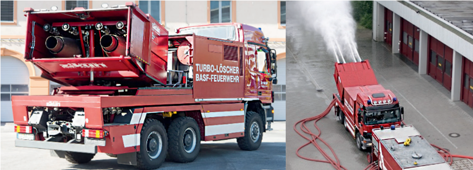
Figure 7: Turbo-reactive extinguisher applied in 2005 by BASF
