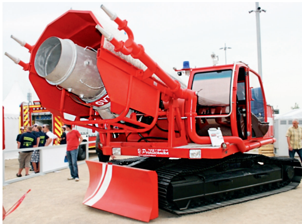
Figure 2: Turbo-reactive extinguisher manufactured by Russian Pozhtehnika
