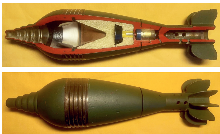
Figure 1–2: 82 mm Soviet shrapnel mortar shell engraving
