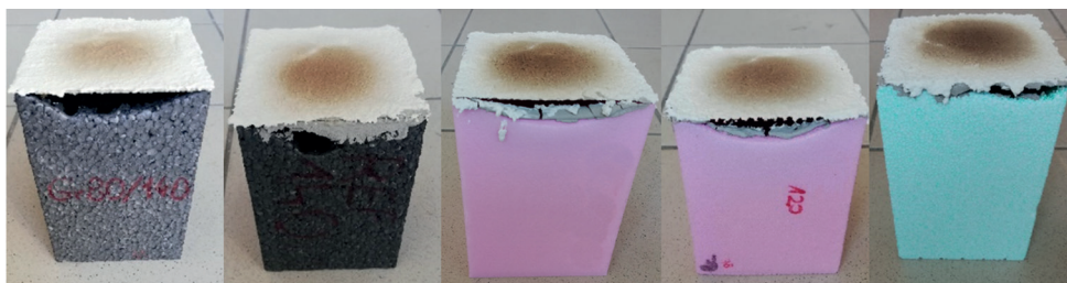
Figure 3: Plastered specimens after test – from left to right GPS-V1-2, XPS-V1-3 Source: compiled by the author
