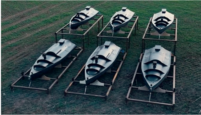
Figure 2: Explosive Uncrewed Surface Vessel (USV)
