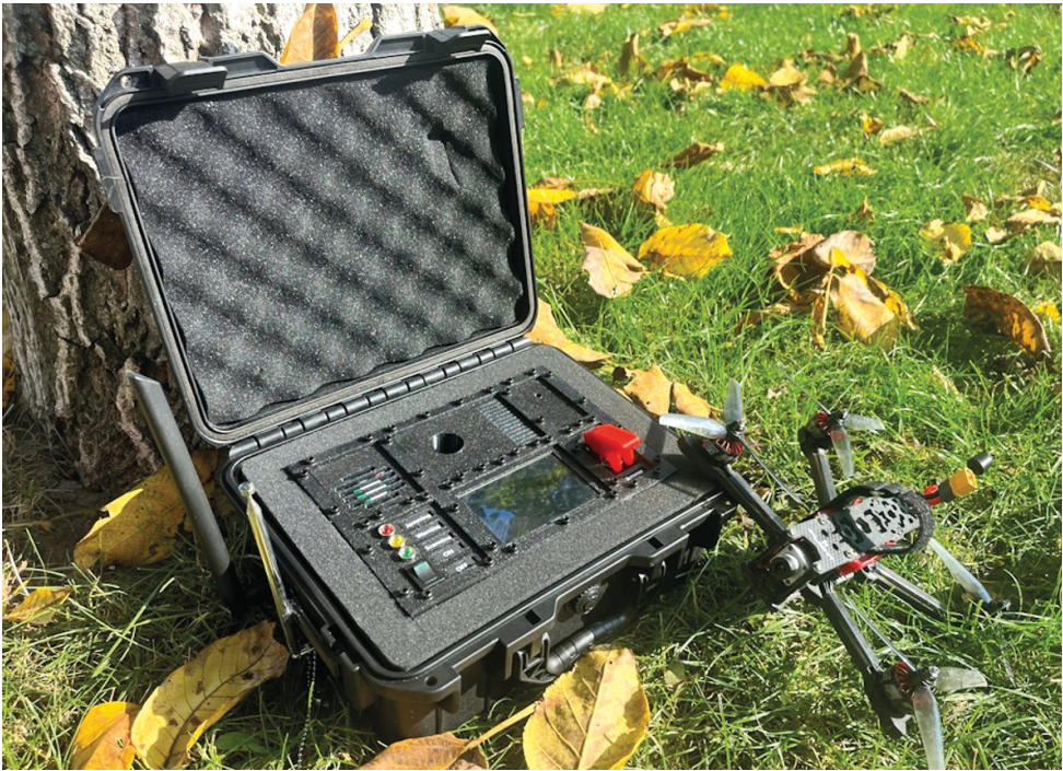
Figure 4: Realised EW platform in a rugged enclosure for field testing
