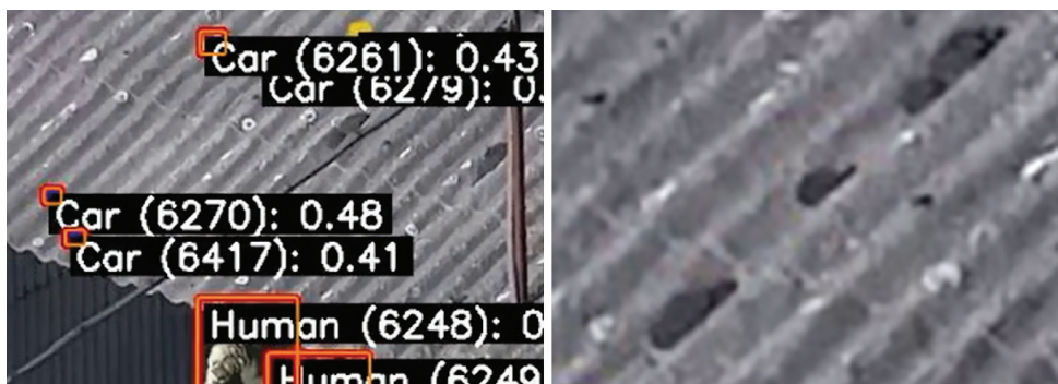
Figure 9: Example of false positive instances on roof with a texture
