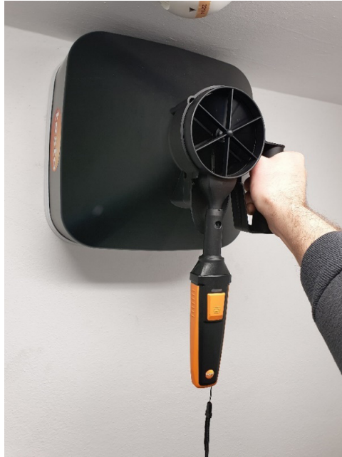
Figure 2: Measurement with funnel vane probe
