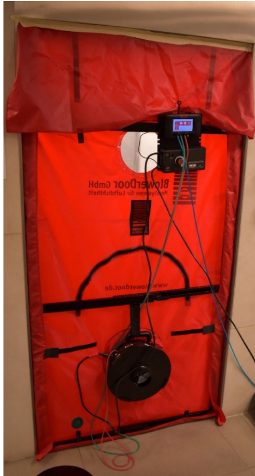
Figure 1: Blower Door instrument installed in a door frame
