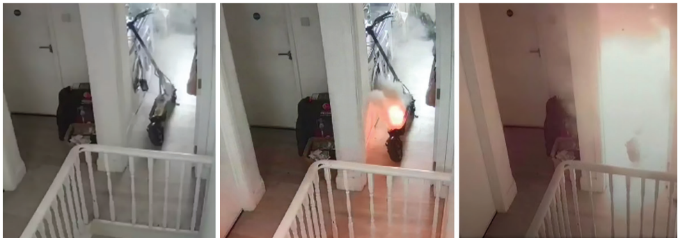
Figure 5: Electric scooter being charged catches fire before exploding Source: London Fire Brigade 2023
