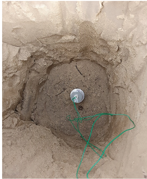
Figure 4: A charge placed in the blasting hole
