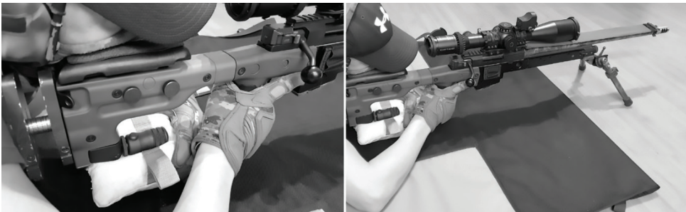
Figure 16: Method No. 7 – Front support (standard tactical bipod, 45° leg angle, resting on concrete surface – hard rubber leg end plug). Rear support (rice filled standard rear bag).
