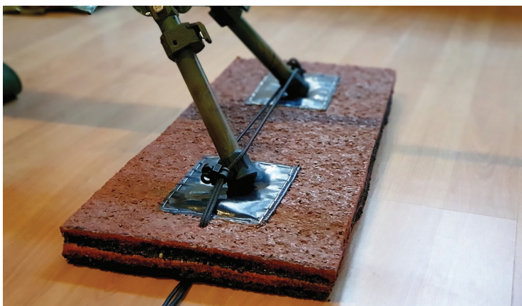
Figure 9: Bipod feet placed on sand bags integrated in a recortan sheet
