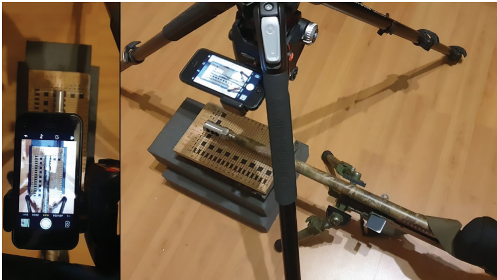
Figure 6: Measuring the recoil distance with a high-speed camera
