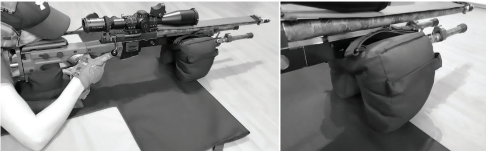
Figure 15: Method No. 6 – Front support (Barricade Bag [~4kg] filled with plastic granules from Cser Ind.). Rear support (eared bag).
