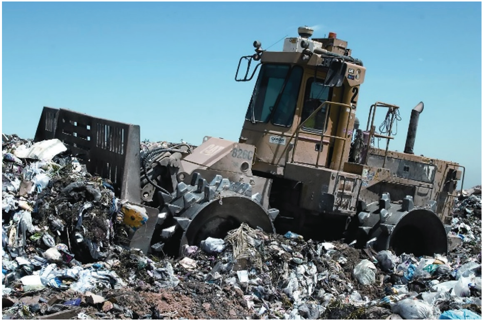
Figure 2: Caterpillar 826C compactor at an Australian landfill
