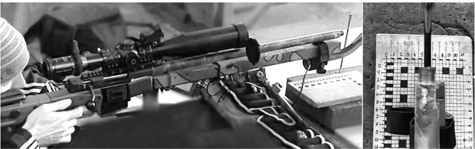
Figure 18: Method No. 9 – Without muzzle break. Front support (standard tactical bipod, 45° leg angle, legs resting on sand-filled neoprene bags). Rear support (tilted, passive support resting on eared bag, hand-controlled monopod).
