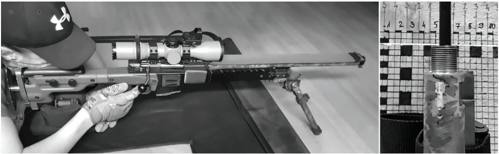
Figure 17: Method No. 8 – Without muzzle break. Front support (standard tactical bipod, 45° leg angle resting on concrete surface – hard rubber leg end plug). Rear support (tilted, passive support resting on a rice-filled rear eared bag, hand-controlled monopod).
