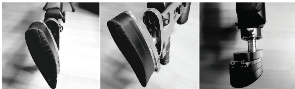
Figure 5: Adjustable butt plate – Accuracy International rubber butt end and a 4-way-adjustable butt plate bracket from a Canadian manufacturer
