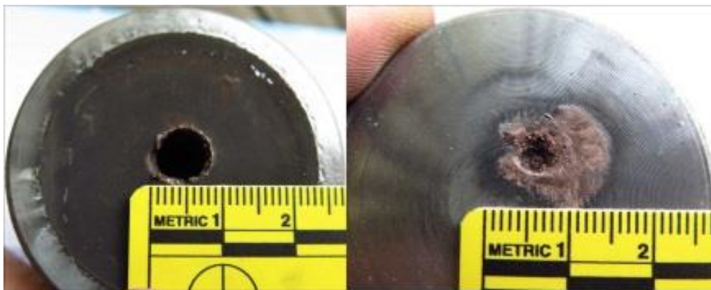
Figure 7: Pressed RDX charge entry (left), and the jet on the second disc (right).
