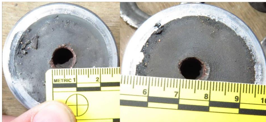
Figure 5: Result for Semtex 1A with (right), and without waveshaper (left)
