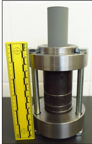
Figure 3: Target assembly with a shaped charge on the top
