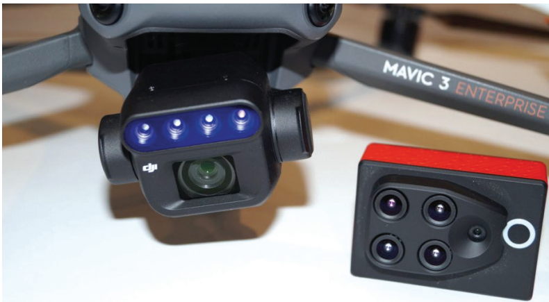
Figure 2: DJI M3M and Parrot Sequoia multispectral cameras
