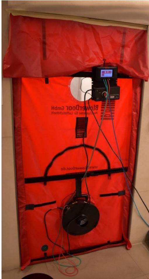
Figure 1: Blower Door instrument installed in a door frame
