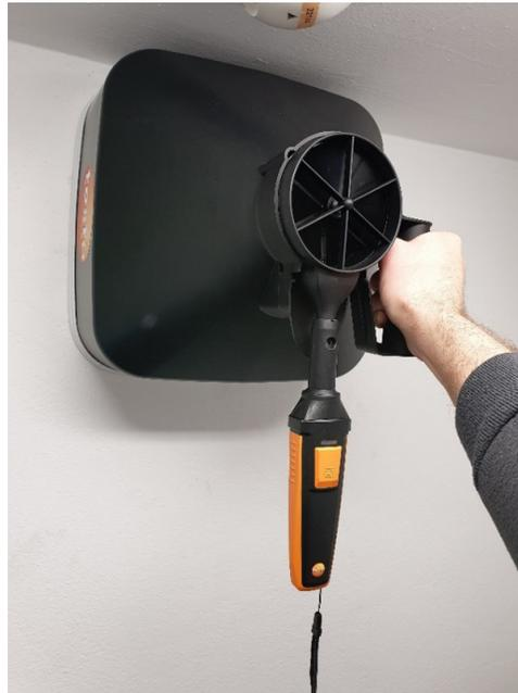
Figure 2: Measurement with funnel vane probe
