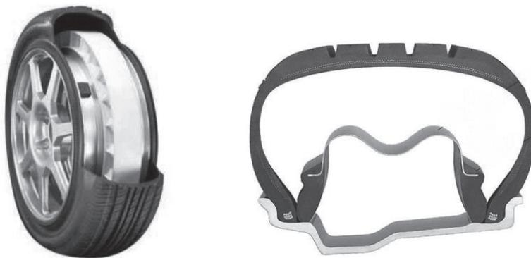
Picture 8. *Run-flat tire with support ring.* [29]
