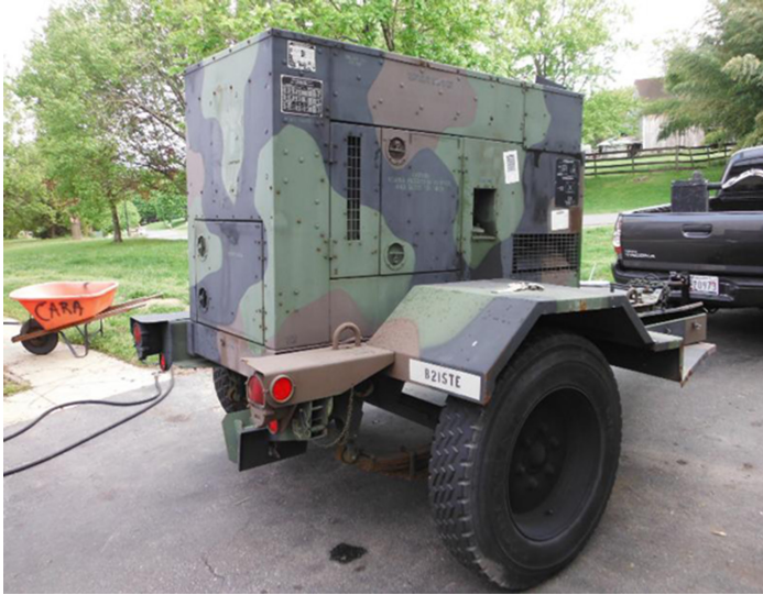
Figure 3. US MEP–805A 3 tons towed military generator driven by a John Deere 4 strokes diesel engine. Max output is 30 kW AC. It has EMP proof capability and quiet working method for tactical missions. [18]
