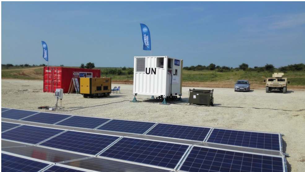
Figure 8. The equipment of Dutch ESTechnologies operating on CL15 exercise in Várpalota supplied a battalion-size camp. 30 [The author's photo.]
