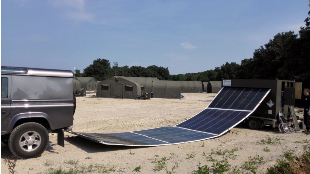
Figure 9. The theory of the British Renovagen is very special and compact. The trailer contains the retractable solar-carpet and the inverters. The tractor Land Rover helps the quick deploy.
