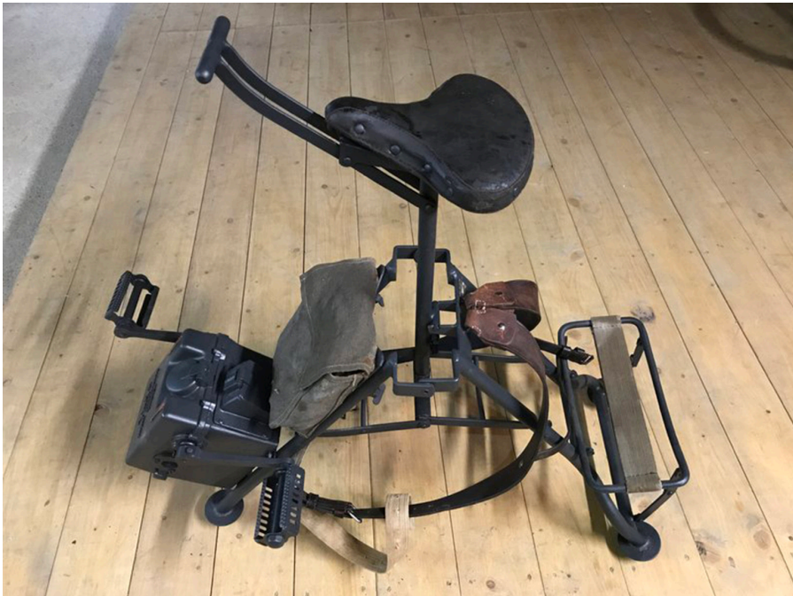
Figure 1. German TP5 pedal-generator before WW2. [17]
