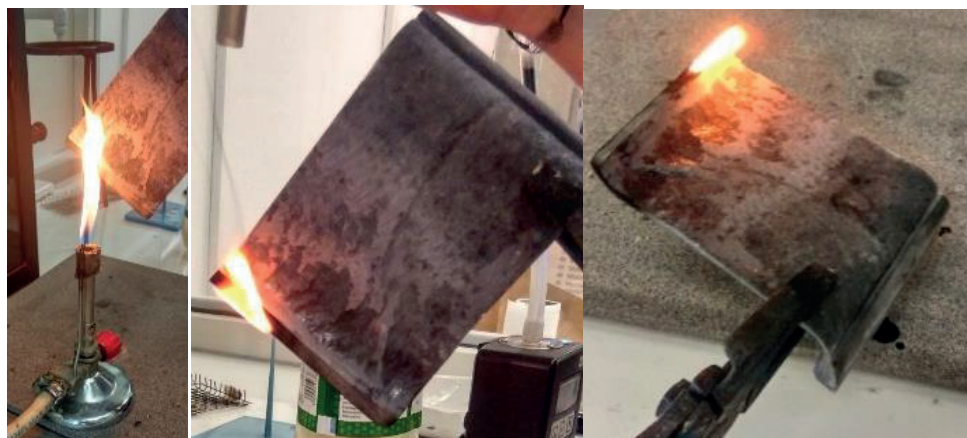
Figure 7: Investigated sample placed to ignition source
