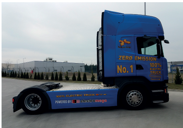
Figure 1: Electrically propelled heavy goods vehicle
