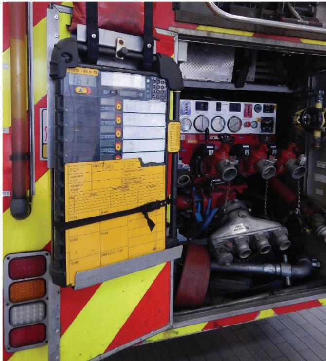
Picture 14: A Draeger Merlin system installed in a fire engine in Liverpool, United Kingdom
