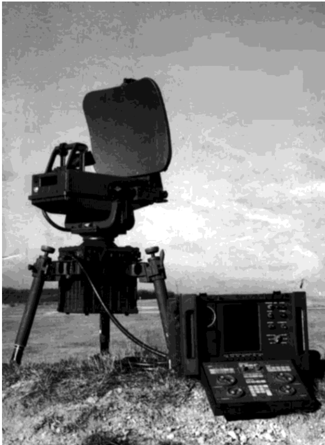
Picture 2. The RATAC reconnaissance radar station, used for the detection and display of enemy tanks and armoured combat vehicles. [5: 75]
