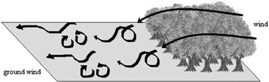
Figure 1. Formation of mechanical turbulence.
